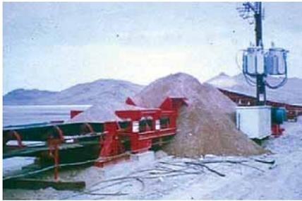
Fig. 4: Plugging and spillage
