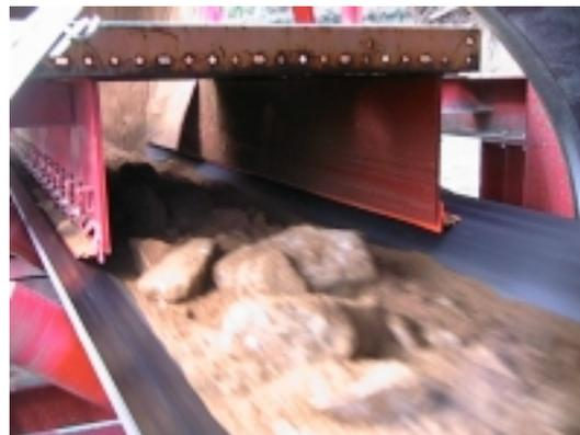
Figure 23 – Material on the receiving conveyor coming right out of one of the transfer stations.
