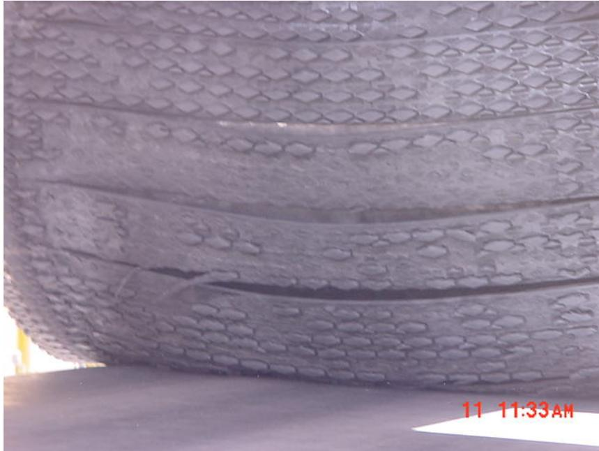
Figure 1 – Picture of a failed lagging application showing both lagging abrasion and delamination
